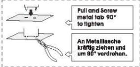
Pull and screw metal tab 90° to tighten
