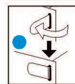
▲ Insert tab and twist 90 degrees is best in some areas to ensure a tight connection
